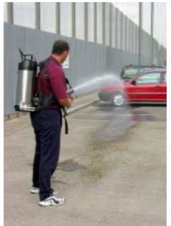
FIGURE 5: Portable Water Cannon
